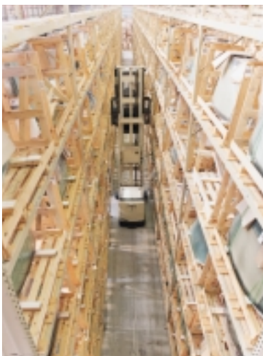
Pilkington AGR Narrow aisle XL racking, fitted with timber shelves and compartments, for the protective storage of car windcreens and windows
